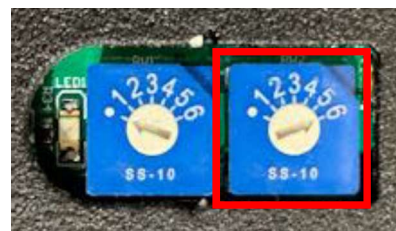
Figure 6 Right Rotary Switch for Off Delay Applications outlined in RED.
