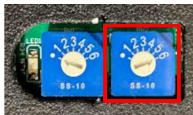
Figure 7 Right Rotary Switch for Off Delay Applications outlined in RED.
