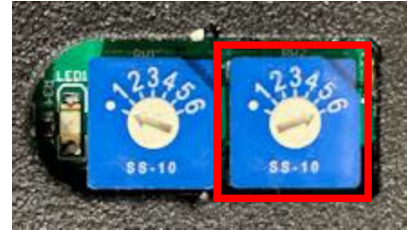
Figure 15 Right Rotary Switch for Off Delay Applications outlined in RED.
