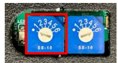
Figure 6 Left Rotary Switch for Measured Voltage Applications outlined in RED.
