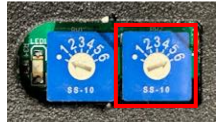
Figure 7 Right Rotary Switch for Off Delay Applications outlined in RED.
