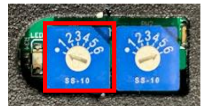
Figure 5 Left Rotary Switch for Measured Voltage Applications outlined in RED.
