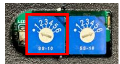
Figure 5 Left Rotary Switch for Measured Voltage Applications outlined in RED.
